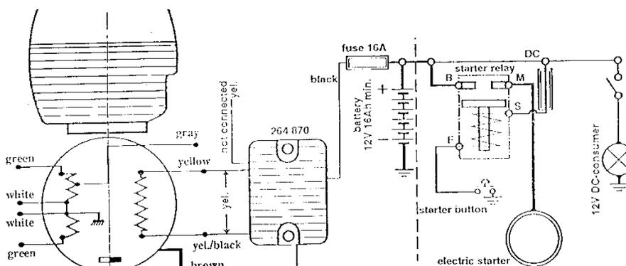
Figure #5 - Illustrates the charging of a battery and the electric start system. Note the extra wire on the regulator is not connect unless desired for back-up.
