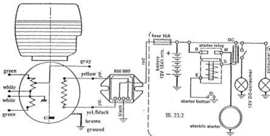
Figure #3 - A typical schematic for using a #9103 single phase regulator to charge a battery and electric start system.
