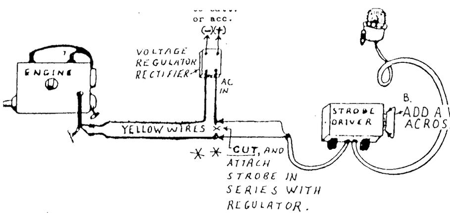
devices to the same set of alternator wires usually brings compatibility problems. In the case of the new Ducati systems there is only one circuit available, forcing you to make some compromises. The simple schematic shown here illustrates how one strobe manufacturer was able to get around this situation. This was accomplished by a redesign of the strobe's circuit by using only the "spare voltage" the regulator did not use.
