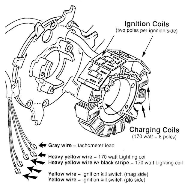
With either system you must realize that this output has it's shortcomings in it's unaltered form. To put it in layman's terms, it's real quite filthy!! Besides being variable by RPM ranging from 6 to 60 volts complete with random voltage spikes, the wave is inconsistent, and the emission of RF waves disrupting radio communication are all present. We obviously need to clean this up before it can be used for just about anything.
